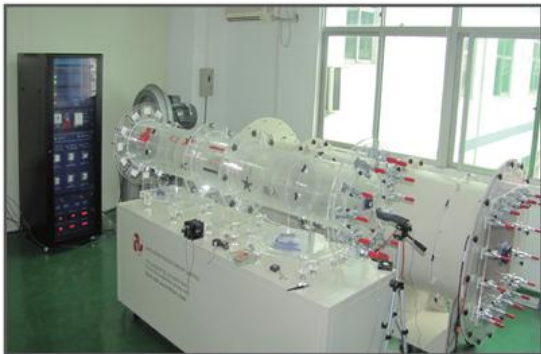
风动测试仪 (CFM test system) Can get the CFM data, mmH 2 O data, working Curve autoly.
