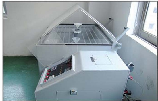
盐雾测试仪 (Salt mist testing system) Test the salt mist performance of Waterproof fan with level IP55 and IP68
