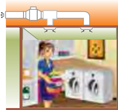
双口横装 Horizontal installation with two diffusers
